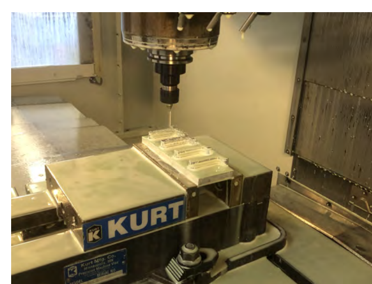
CNC Milling Custom Clamps
