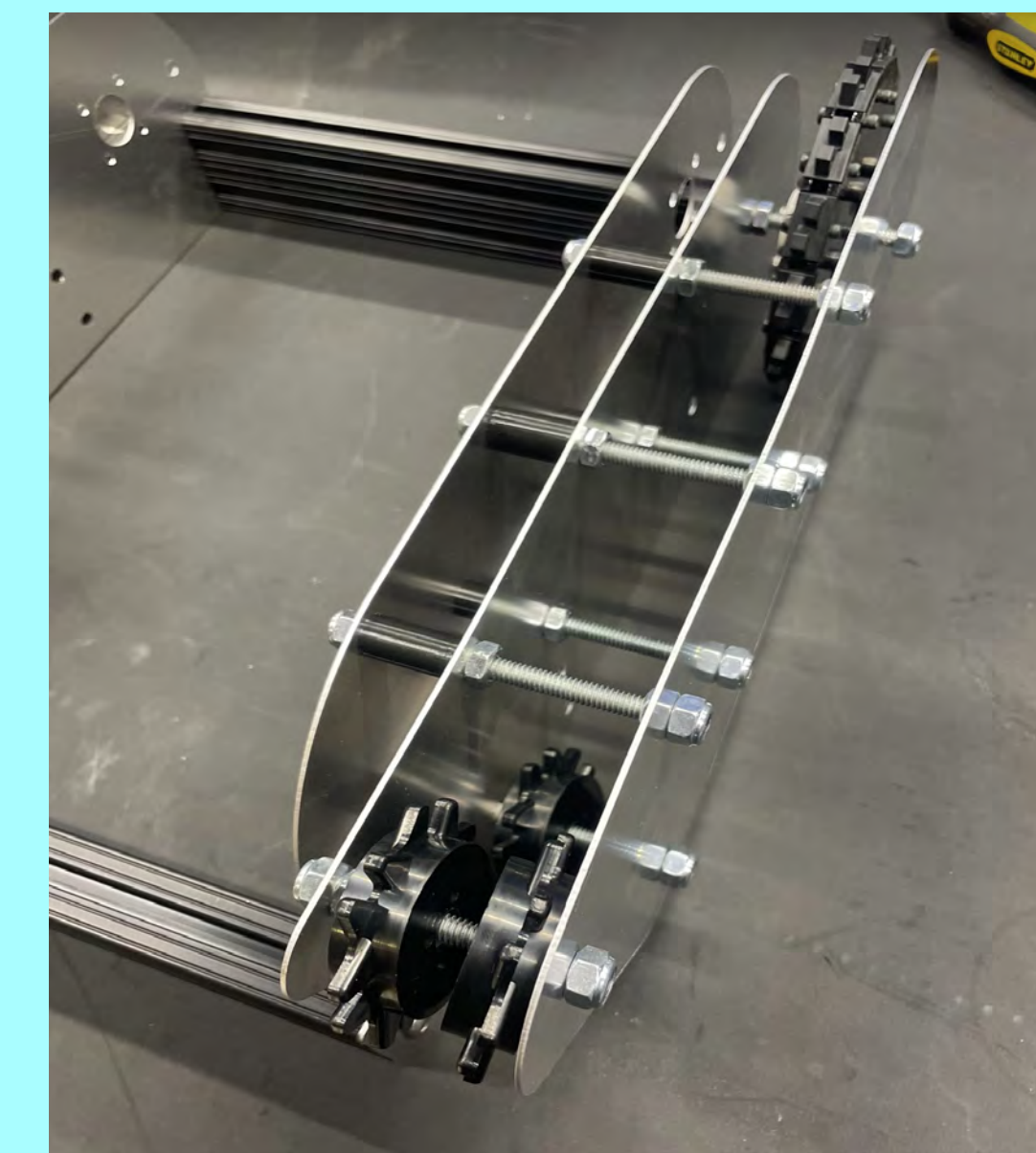
Assembling Drivetrain Tracks
