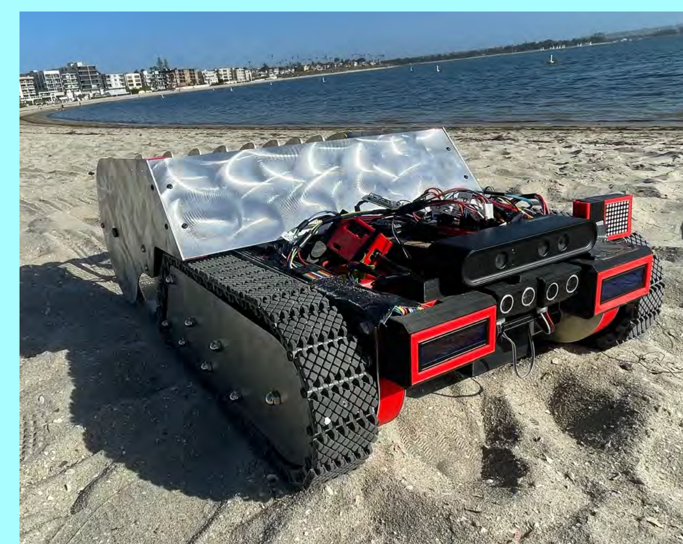
Beach testing of tank tracks, collection system, and total electronics integration
