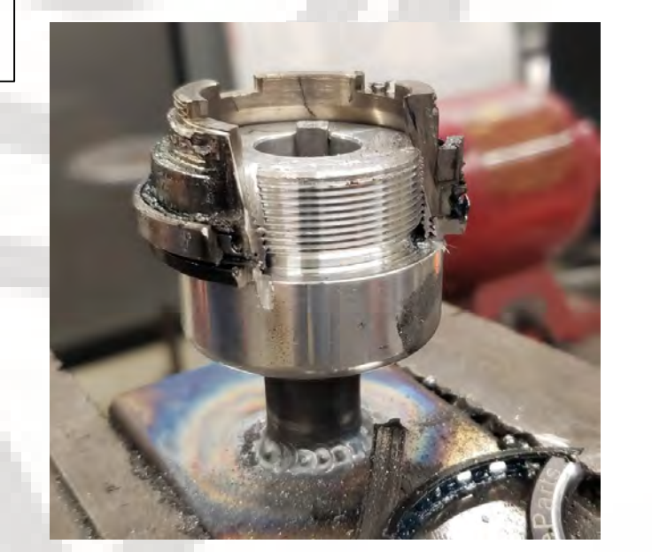
Torque Test for Sprag Gear
