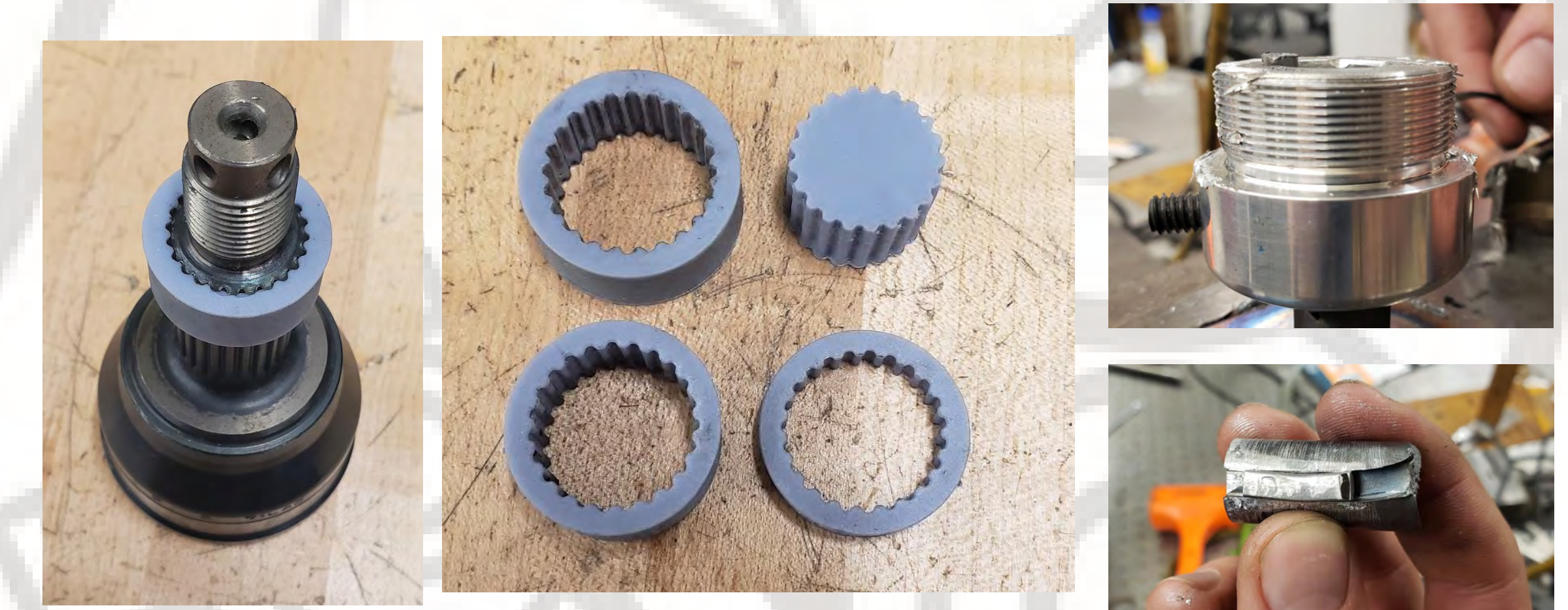
Fitment Test of the CV Spline
